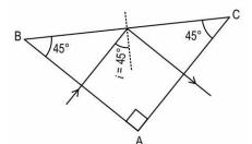
Find the minimum value of refractive index n of the prism required for the total internal reflection of the light to occur on the face BC of the prism.
